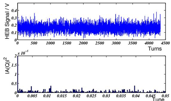
Figure 8: Top: HEB signal of single bunch with a low bunch current for about 4100 consecutive revolutions (top) and its FFT (bottom). No significant features are seen.
