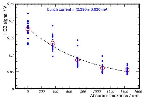
Figure 6: HEB signal as function of absorber thickness. The red circles represent the average of the dataset for each absorber thickness. The dashed curve is the result of an exponential fit to the data.
