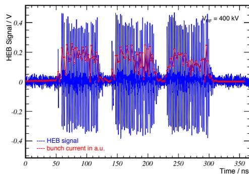
Figure 5: HEB signal for a different set of accelerator parameters ( $E_0 = 1.3 \text{ GeV}$ ,  $V_{\text{RF}} = 400 \text{ kV}$ ) resulting in shorter bunches and an increased power of the THz signal (blue). The red data curve shows the relative bunch currents. For large currents the HEB signal shows clear signs of saturation, i.e. it becomes largely independent of the bunch current.
