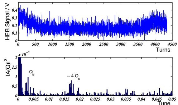
Figure 7: HEB signal of single bunch with a high bunch current above the bursting threshold for about 4100 consecutive revolutions (top) and FFT of signal (bottom). The frequency spectrum shows the synchrotron tune and the fourth harmonic of the synchrotron tune.
