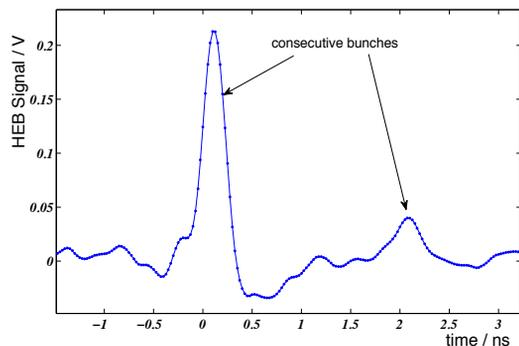
Figure 2: Hot electron bolometer signal as a function of time showing in high resolution two consecutive bunches of different current in the MLS. The resolution of the bunch length is in this case limited by the bandwidth of 2.5 GHz of the oscilloscope used for the measurement. The FWHM of the signal from the readout electronics of the bolometer is 165 ps.
