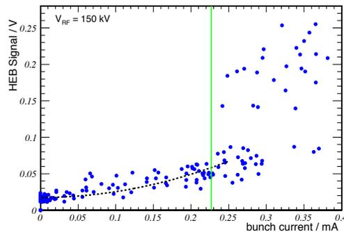
Figure 4: HEB signal of Fig. 3 as a function of the corresponding single bunch current. The line marks the expected bursting threshold for the given accelerator parameters. The dashed curve, a fit of a quadratic dependence on bunch current to the measurements, was added to guide the eye.
