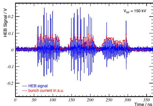
Figure 3: HEB signal showing clearly the filling pattern in the ANKA storage ring (blue). The red data points represent the relative bunch currents derived from the sum signal of four button electrodes. In order to have as broad a range in bunch currents as possible, a very inhomogeneous filling pattern was enforced.
