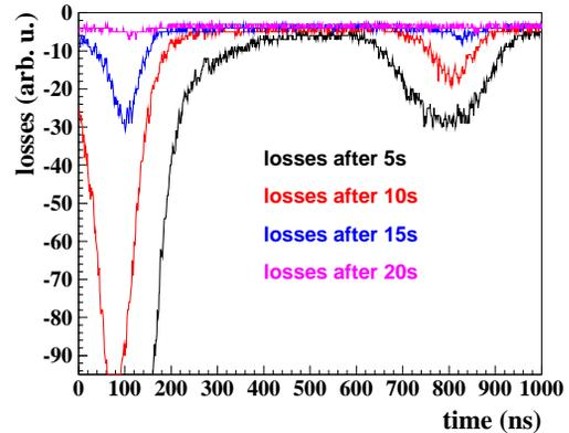
Figure 6: Losses of the accumulated and damped beam when powering the kickers with a frequency of 0.2 Hz. All data correspond to a single filling.
