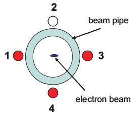
Figure 2: Position of the glass fibers as installed at the MLS. Fiber 1 is located at the inside of the ring. Due to the small vertical aperture the symmetric geometry as depicted in the graph could not be realized within the dipole magnets and the undulator.
