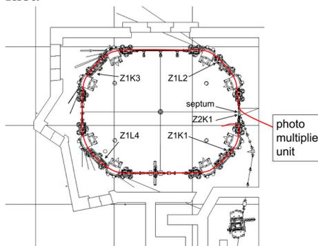
Figure 1: Arrangement of the Cherenkov fibers (red) and the foil monitors at the MLS. The undulator U180 is installed in the straight between Z1L2 and Z1K3.
