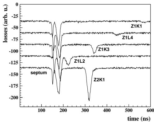
Figure 4: Losses of a short bunch at various foil monitors. The shower at FOM Z2K1 (upstream of the injection straight) does not hit the end of the fiber since it is already bent to the inside of the ring but the fiber part at the septum.
