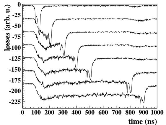
Figure 3: Injection of bunch trains of different lengths. The beam is intentionally dumped with a foil monitor at the septum.
