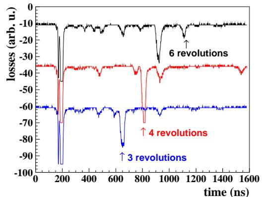
Figure 7: Electron losses at the septum after 6, 4 and 3 revolutions in the storage ring for horizontal tunes of 0.185 (black), 0.256 (red) and 0.320 (blue).
