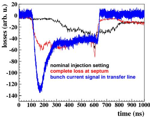
Figure 5: Losses for nominal injection conditions (black) and best transmission (red). For comparison the charge distribution as measured with a stripline upstream of the septum is plotted (blue).
