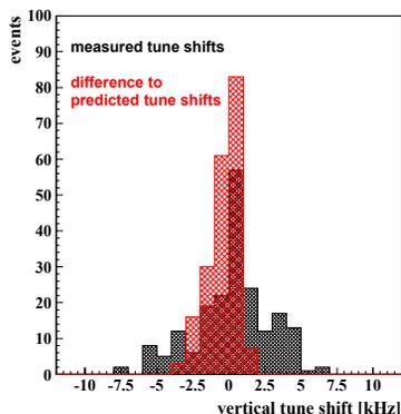
Figure 5: Measured vertical tune shifts (black) and deviation to simulation (red) of the BESSY II UE112.
