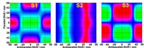
Figure 2: Contour plot of the Stokes parameter S1, S2 and S3 versus the phase parameters  $pp \times \lambda$  (vertical axis) and  $pa \times \lambda$  (horizontal axis).
