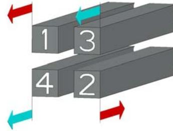
Figure 1: The variables  $pp$  (blue) and  $pa$  (red) define the distance of parallel motion (rows 3, 4) and antiparallel motion (rows 1, 2), respectively. The device is operated with an arbitrary combination of  $pp$  and  $pa$ .
