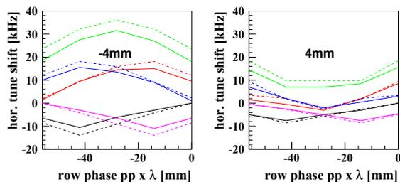
Figure 3: Horizontal tune shifts of the BESY II UE112 versus row phase  $pp$  as defined in figure 1. The colours correspond to values of  $pa = 0$  (black), 0.125 (red), 0.250 (green), 0.375 (blue), 0.500 (magenta). Solid lines: measurements, dashed lines: simulations.
