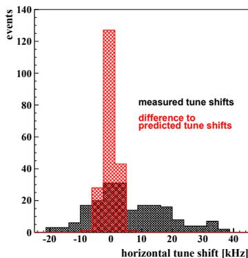
Figure 4: Measured horizontal tune shifts (black) and deviation to simulation (red) of the BESSY II UE112.
