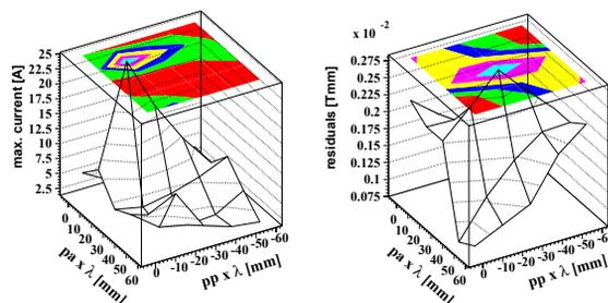
Figure 6 (left): Maximum compensation currents. Figure 7 (right): Residuals of field integrals with compensation for various combinations of  $pp$  and  $pa$ .
