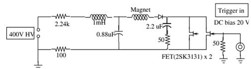
Figure 4: Schematic view of developed drive circuit.
