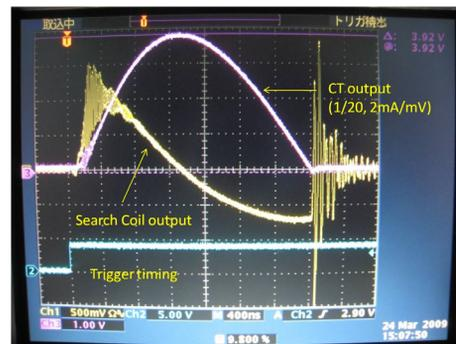
Figure 5: Output signal of S.C. and CT probe in synchronized with trigger timing.
