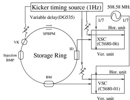
Figure 1: Overview of the experiment system.
