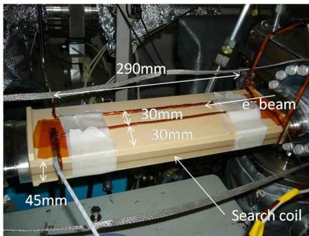
Figure 2: Setup of vertical kicker.
