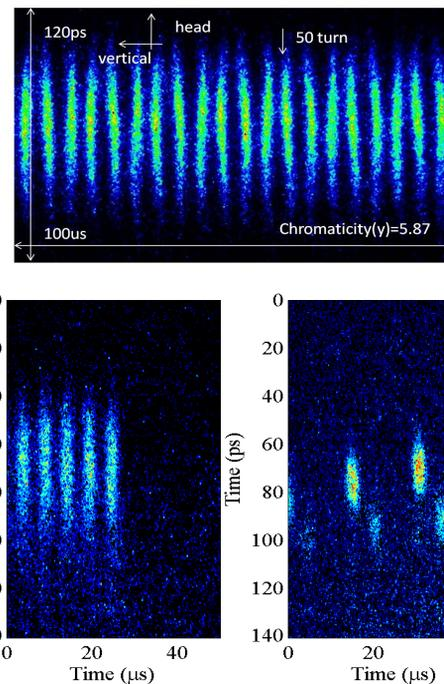
Figure 6: Upper picture shows the profile observed by VSC. Lower figures show the profiles observed by XSC after slit slicing in kicker OFF (left) and kicker ON (right).
