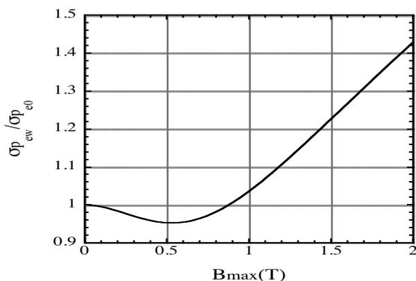
Figure 4: Relative momentum deviation as a function of maximum wiggler fields. Total wiggler length is 120 m.
