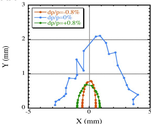
Figure 2: Dynamic aperture at the center of short straight section.
