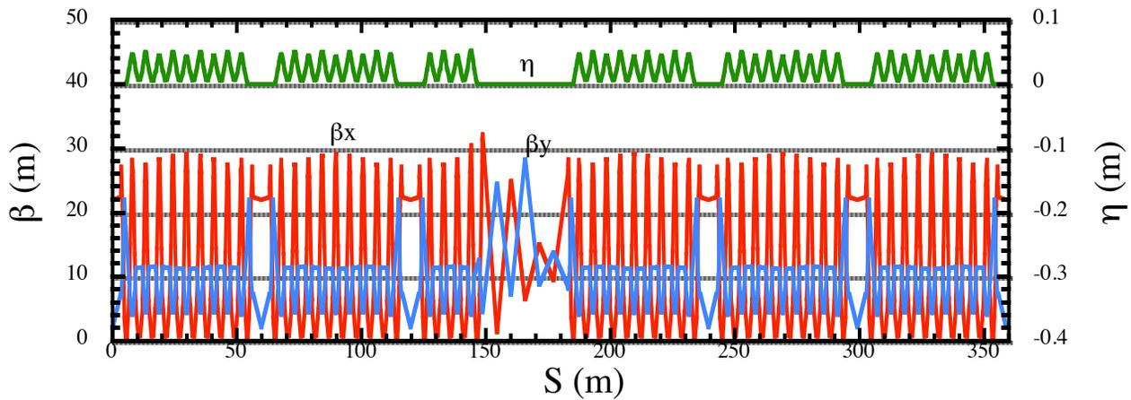
Figure 1: Optics functions in one-quarter of storage ring.
