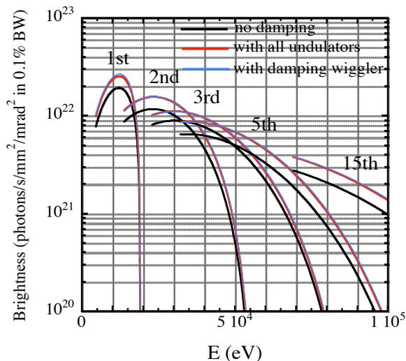
Figure 5: Brightness for a 4.5 m undulator with no damping, damping by undulators, and damping by wigglers.
