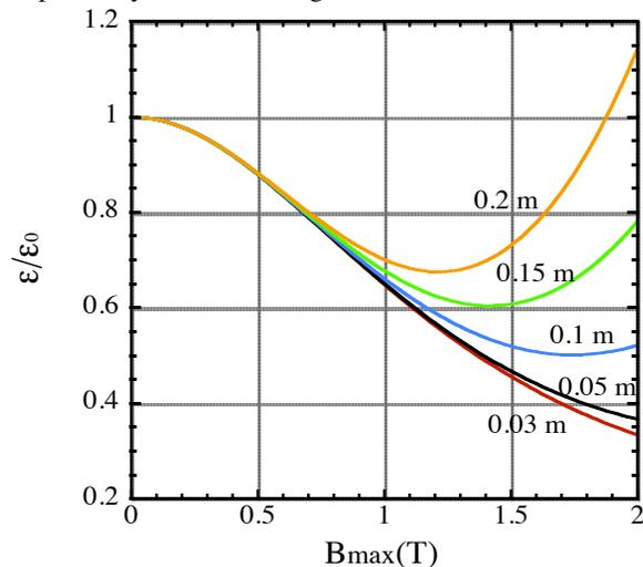
Figure 3: Emittance reduction by damping wigglers: 0.2m, 0.15 m, 0.1 m, 0.05 m, and 0.03 m period wigglers.
