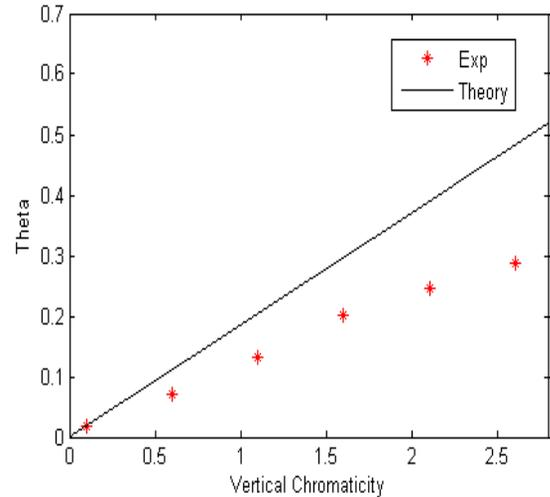
Figure 6: Tilt angle in rad vs. chromaticity
