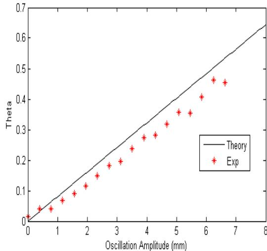
Figure 5: Tilt angle in rad vs. oscillation amplitude.
