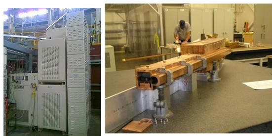
Figure 1: Example of newly installed or upgraded hardware: New booster bend magnet power supply; upgraded septum magnet.
