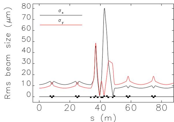
Figure 2: Test of the rotation system and triplet relay optics.
