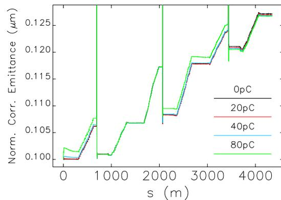
Figure 5: Evolution of horizontal emittance in the presence of CSR for four bunch-charge levels.
