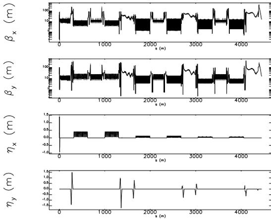
Figure 3: Optics of entire system, with x-y rotators off.
