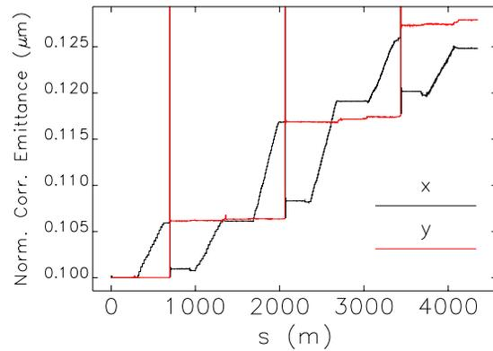
Figure 4: Evolution of the emittance in the presence of synchrotron radiation. Off-scale spikes indicate the locations of the x-y rotators.
