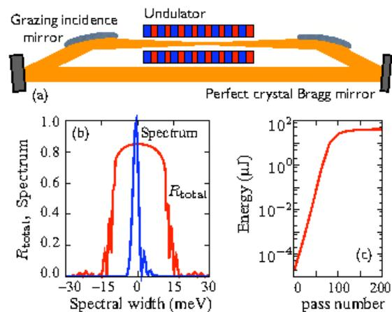
Figure 1: Panel (a) shows a schematic of the FEL oscillator in near-backscatter geometry. Panel (b) shows the bandpass of the diamond mirror near 12-keV (red) and the saturated radiation spectrum (blue) that is transmitted through the thin mirror. These spectra are representative of the various parameters listed in Table 1. Panel (c) shows the initial exponential gain for the 12 keV oscillator, with saturation after 50-200 passes being typical for the FEL configurations listed in Table 1.
