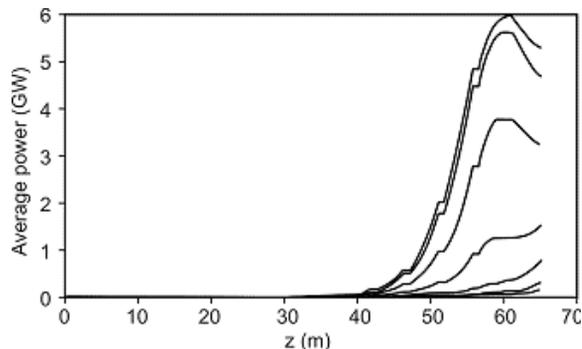
Figure 6: Power growth curves for the beam centroid initial offsets ranging from 0 to  $3\sigma$ .
