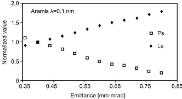
Figure 3: The normalized saturation length (Ls) and power (Ps) dependence on the beam emittance.
