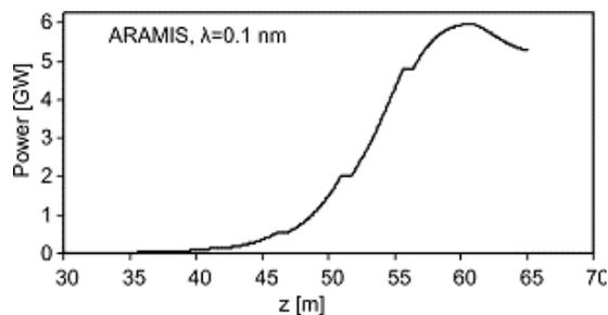
Figure 2: The Aramis SASE FEL power growth curve for beam design parameters.
