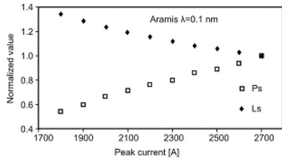
Figure 5: Normalized saturation length (Ls) and power (Ps) dependence on the beam peak current.
