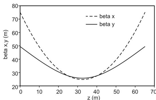
Figure 8: The horizontal and vertical beta functions in Aramis undulator line.
