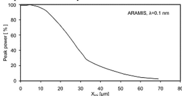
Figure 7: Radiation peak power reduction due to initial spatial offset in Aramis undulator.
