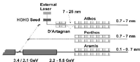
Figure 1: Schematic layout of PSI-XFEL undulator lines.
