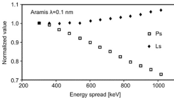
Figure 4: Normalized saturation length (Ls) and power (Ps) dependence on the beam energy spread.
