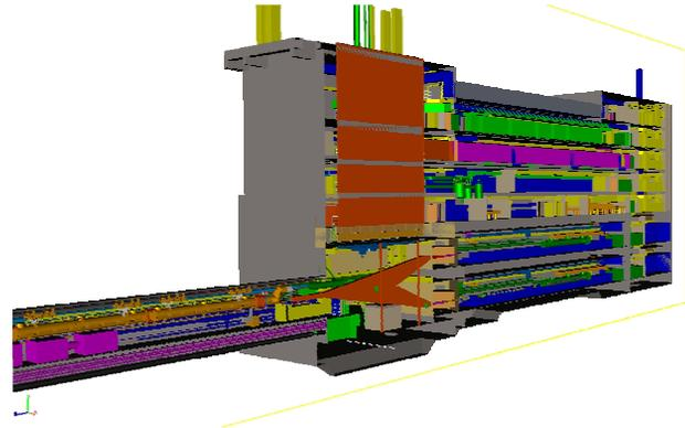
Figure 1: Model of the injector shaft, showing the tight interconnections of civil construction, technical infrastructure and accelerator.
