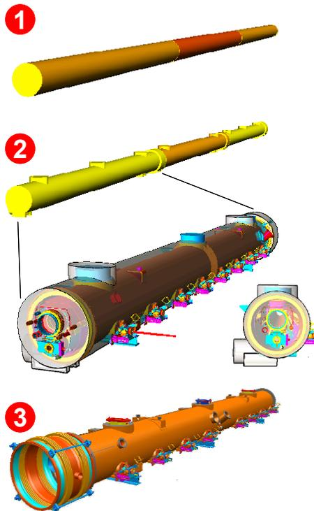
Figure 6: Lattice (1), accelerator made up of placeholders (2) and detailed component models (3). Placeholders link and decouple component design and facility planning.
