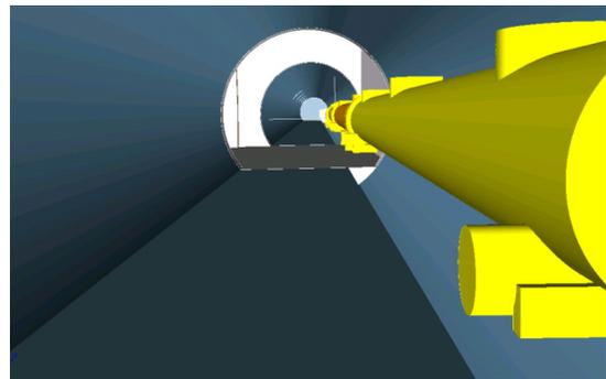
Figure 5: Prototype model of the ILC containing tunnel segment, cavern and shaft and the main linac, positron source and beam delivery systems.
