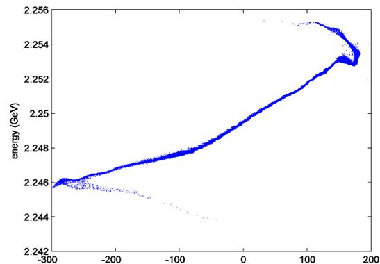
Figure 3: Typical longitudinal phase space plot of the electron beam at the exit of the LINAC.
