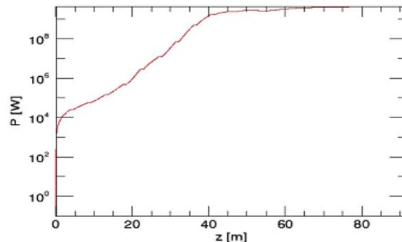
Figure 5: FEL power as a function of the distance travelled in the undulator train. GENESIS time dependent simulations.
