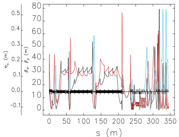
Figure 2: Twiss parameters for the LINAC, collimation, diagnostics and spreader sections.
