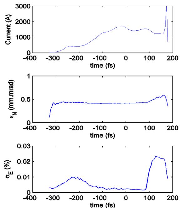
Figure 4: Typical electron beam slice parameters at the exit of the LINAC.
