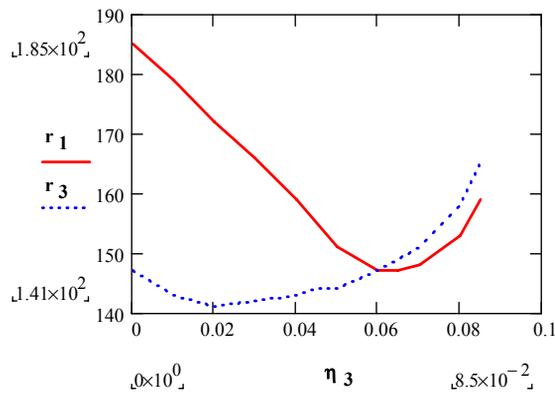
Figure 5: Round trip number needed to reach the saturation for the fundamental ( $r_1$ ) and for the 3rd harmonic ( $r_3$ ) vs.  $\eta_3$ .
