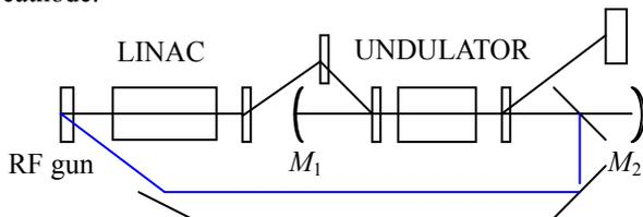
Figure 1: Layout of a self sustained FEL device.
