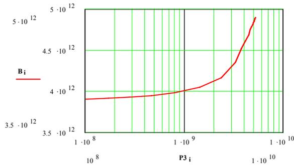
Figure 4: e-beam brightness ( $A\ m^{-2}\ rad^{-2}$ ) vs. the illuminating power ( $W\ m^{-2}$ ).
