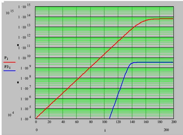
Figure 3: The intra-cavity round trip evolution ( $W/m^2$ ) of the fundamental (red) and the 3rd harmonic (blue) at  $\eta_3=0$ .
