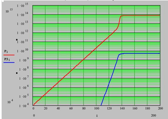
Figure 2: The intra-cavity round trip evolution ( $\text{W}/\text{m}^2$ ) of the fundamental (red) and the 3<sup>rd</sup> harmonic (bleu) at  $\eta_3=6\%$ .
