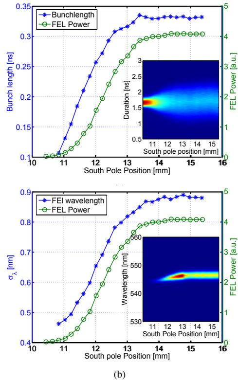
Figure 4: (a) The bunch length and FEL power as a function of the south pole position; (b) The FEL bandwidth and FEL power as a function of the south poles position. All other three poles are parked in the fully open positions. The FEL and electron beam parameters are the same as in Fig. 3. In the insets, the bunch longitudinal profiles and FEL lasing spectra are re-plotted as intensity plots.
