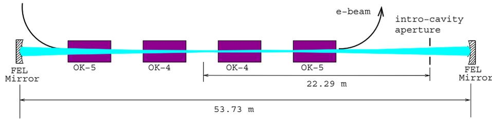
Figure 1: The layout of the Duke FEL oscillator cavity.
