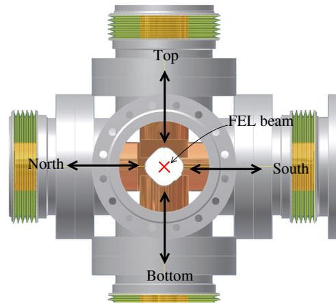
Figure 2: The front view of the water-cooled in-cavity aperture system.
