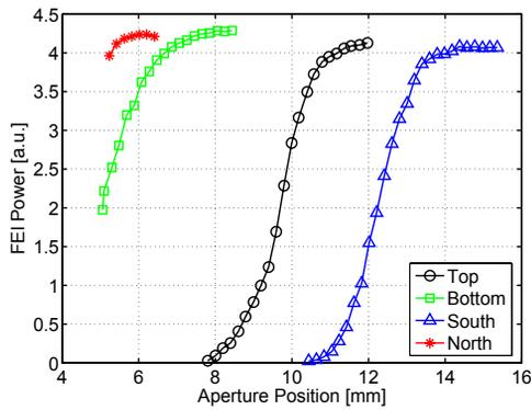
Figure 3: The extracted FEL power during the scanning of the aperture poles. The two-wiggler OK-5 FEL is lasing at 545 nm with a single-bunch current of 20 mA and an electron beam energy of 435 MeV.
