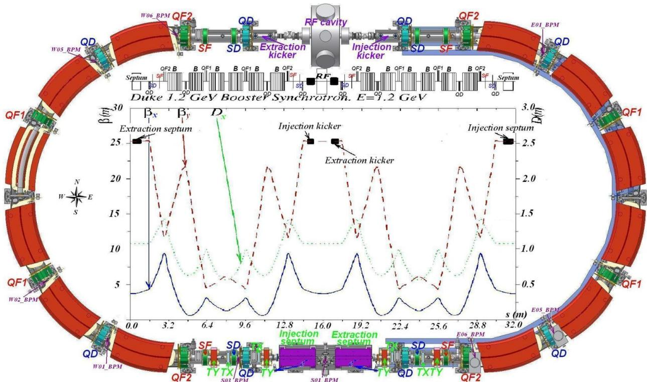
Figure 1: Mechanical layout and magnetic lattice of the Duke booster synchrotron.
