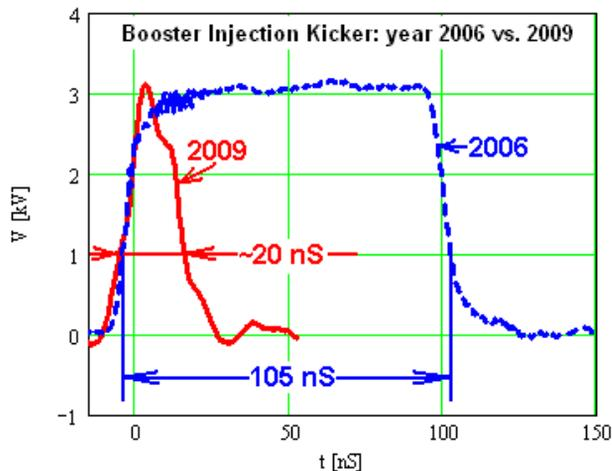
Figure 2: Injection kicker pulse before and after modification of the driver. Voltage per one electrode.
