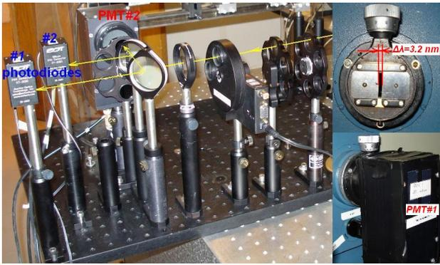
Figure 1: A four-stage FEL gain measurement bench with two photodiodes and two PMTs. On the right: the 1<sup>st</sup> stage PMT receives the optical beam after a monochromator with the exit slit opened to about 3.2 nm.
