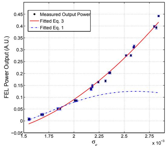
Figure 3: Measured FEL output power as a function of the energy spread of the electron beam. Beam energy is 425 MeV,  $N_d = 31$  and  $N_w = 33$ .
