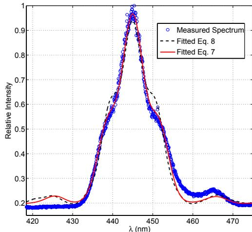
Figure 2: OK-4 spectrum with a single-bunch electron beam. Beam current is 10.61 mA, beam energy is 425 MeV,  $N_d = 31$ , and  $N_w = 33$ . The fit energy spread is  $\sigma_\epsilon = 2.57 \times 10^{-3}$  by the solid curve.
