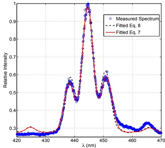
Figure 1: OK-4 spectrum with a single-bunch electron beam. Beam current is 5.87 mA, beam energy is 425 MeV,  $N_d = 31$ , and  $N_w = 33$ . The fit energy spread is  $\sigma_\epsilon = 1.55 \times 10^{-3}$  by the solid curve.
