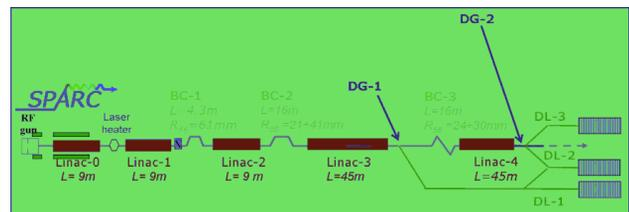
Figure 3: SPARX acceleration and compression schematic layout using SPARC injector.
