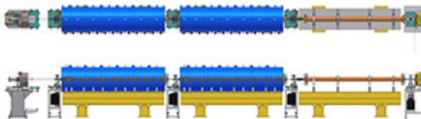
Figure 1: Top and side view of the SPARX Photoinjector.
