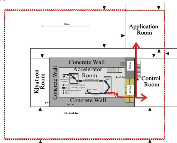
Figure 1: Diagram of KU-FEL facility and MIR-FEL beam transport line.
