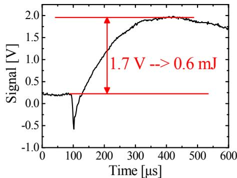
Figure 5: Preliminary measurements for the energy at the experiment room.
