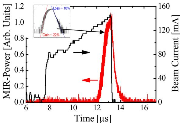
Figure 2: The temporal profile of the beam current and MIR-power
