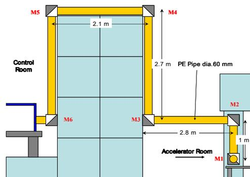
Figure 4: A diagram of MIR-FEL beamline.
