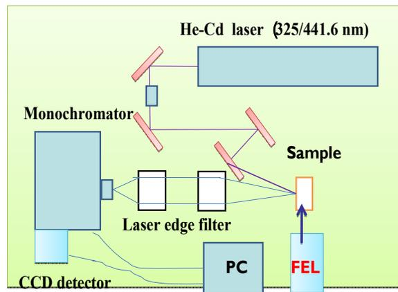
Figure 6: A plan view of optical measurement system by FEL
