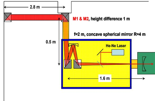
Figure 3: Schematic drawing of the beam expander.
