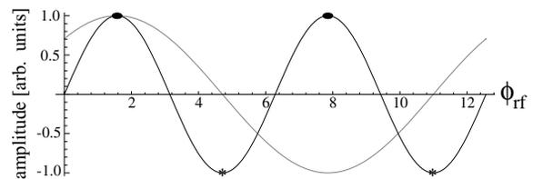
Figure 1: Two bunches (large dots) from two cycles of the main linac wave (black) are synchronized with a subharmonic wave (gray) to accelerate the first bunch and decelerate the second. A few-percent energy separation can be gained in a single-cell subharmonic cavity. Off-crest operation is possible. Energy-recovery bunches (stars) can also pass the subharmonic cavity at the zero crossings for merging three beams. There is little beam loading in the subharmonic cavity.
