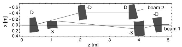
Figure 2: Schematic of a two-beam merger. Going backward, two bunches with 5% energy separation are bent by a 15° dipole (D) into slightly different directions. The high-energy bunch is deflected by a static dipole septum (S) and then passes through a zigzag achromat formed with two opposite dipoles (-S and -D). The low-energy bunch passes through a 3-dipole achromat. With some effort, it may be possible to merge the energy-recovery beam at the same time (not shown).
