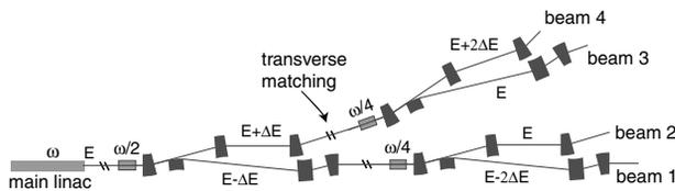
Figure 3: Schematic of a 4-beam merger by staging three 2-beam mergers (the high-energy beam is not shown). The subharmonic frequencies and beam energies are indicated. No pulsed devices (magnetic or rf kickers) are used in the merger to preserve beam emittance.
