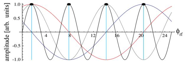
Figure 4: Synchronization of four cavity waves to introduce the required energy separation in adjacent four bunches. Black curve is the main linac wave of frequency  $\omega$ . Gray wave separates bunches 1 and 3 from bunches 2 and 4 at frequency  $\omega/2$ . Red (blue) wave further separates bunch 1 (2) from 3 (4) at frequency  $\omega/4$ .
