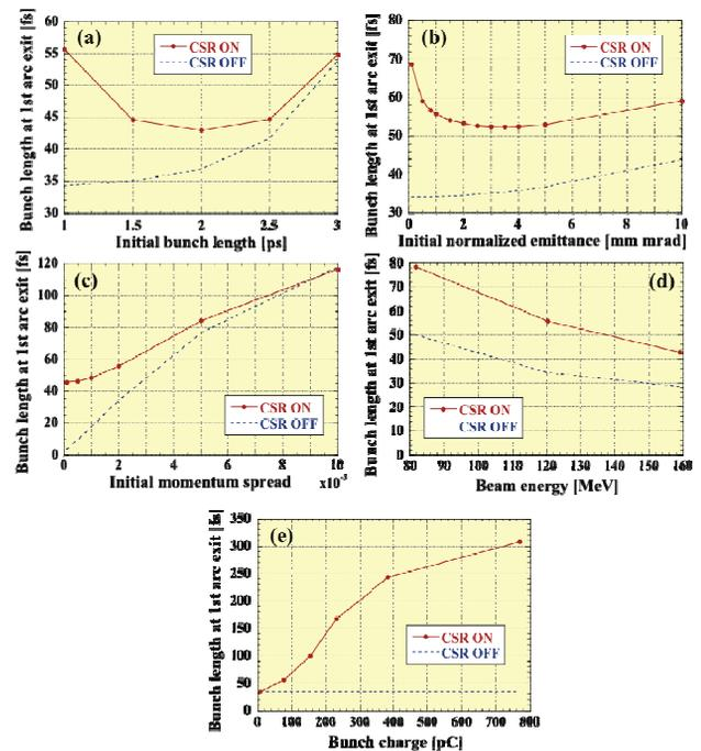
Figure 8: Dependence of bunch length at exit of the 1<sup>st</sup> arc section on (a) initial bunch length, (b) initial normalized emittance, (c) initial momentum spread, (d) beam energy and (e) bunch charge in BC mode.
