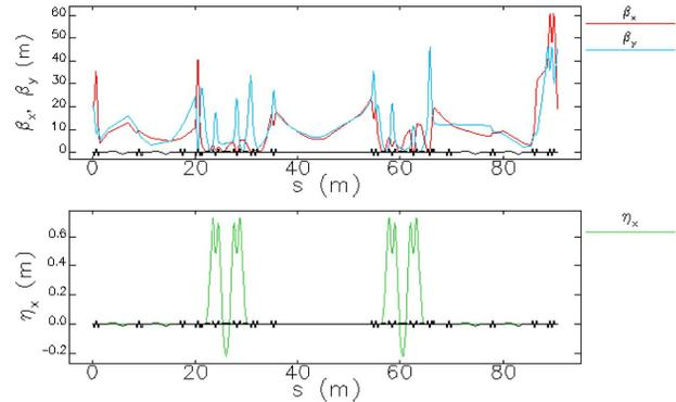
Figure 2: Betatron and dispersion functions of the compact ERL in HC mode.
