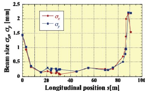
Figure 4: Horizontal and vertical beam sizes along longitudinal position for the initial bunch length of 2ps in HC mode.
