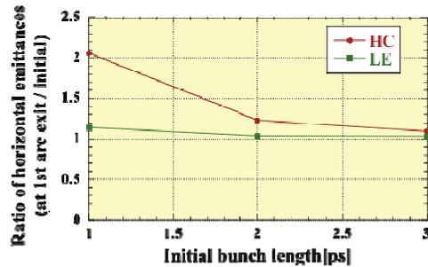
Figure 3: Dependence of normalized horizontal emittance on initial bunch length. The initial emittances are 1 and 0.1 mm·mrad for HC and LE modes, respectively.
