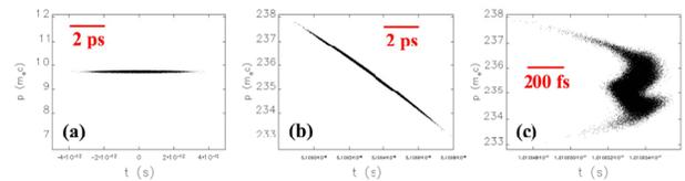
Figure 6:  $(t, p)$  distribution of bunch (a) at initial position, (b) after accelerating RF cavity modules and (c) at exit of 1<sup>st</sup> arc section. Momentum  $p$  is expressed in unit of  $m_e c$ .
