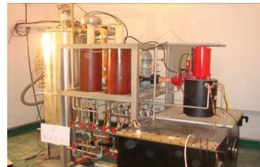
Figure 9: Photo of the 10MeV linac.
