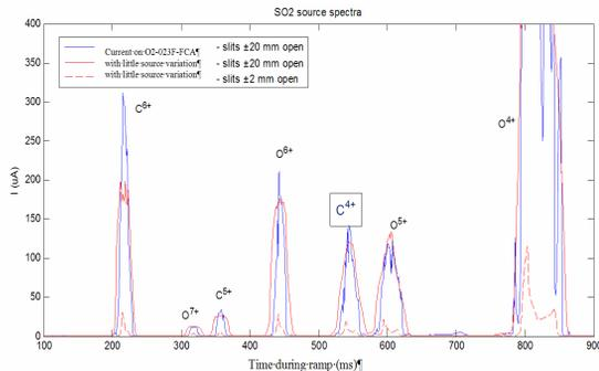
Figure 2: Beam spectra done ramping O2-018A-IDA spectrometer. The signal is acquired on the O2-023F-FCA Faraday cup.
