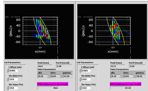
Figure 5: Horizontal (left) and vertical (right) emittance at the RFQ entrance with  $C^{4+}$  beam
