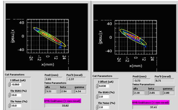
Figure 4: Horizontal (left) and vertical (right) emittance in L1-017B-SLA with  $C^{4+}$  beam.
