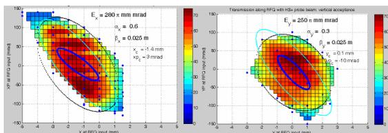
Figure 8: Horizontal (left) and vertical (right) RFQ acceptance measurements done with  $H_3^+$  at 8 keV/u.
