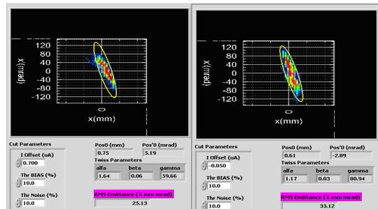
Figure 6: Horizontal (left) and vertical (right) emittance at the RFQ entrance with  $H_3^+$  beam.
