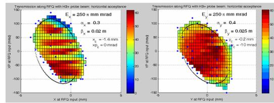
Figure 9: Horizontal and vertical RFQ acceptance measurement done with  $H_3^+$  at 8.5 keV/u.
