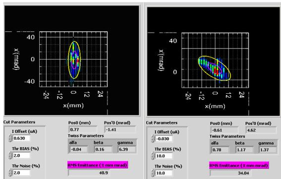
Figure 3: Horizontal (left) and vertical (right) emittance in O2-023B-SLA with  $C^{4+}$  beam.
