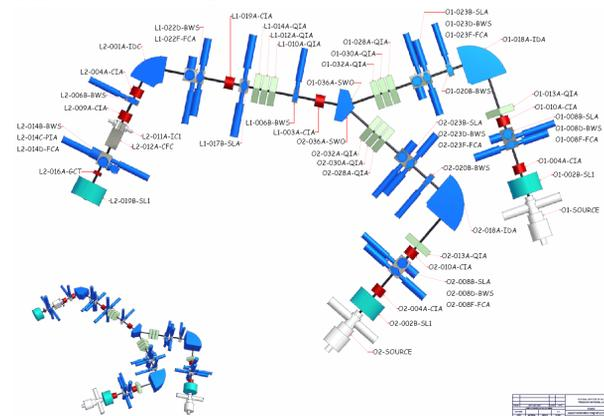
Figure 1: LEBT layout. Magnetic and diagnostic elements of the line are labelled.
