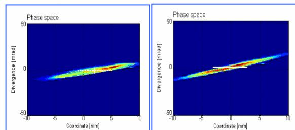
Figure 10: Horizontal (left) and vertical (right) emittance measured in TB2 with  $C^{4+}$  at 8 keV/u.
