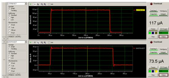
Figure 7: Current signals upstream and downstream the RFQ with  $C^{4+}$  beam at 8 keV/u and setting a non dispersive optics (achromatic) in L2. The beam pulses were formed by the electrostatic chopper in L2.
