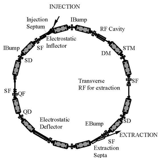
Figure 1: Schematic view of synchrotron. DM: Dipole magnet; QF, QD: Quadrupole magnet; SF, SD: Sextupole magnet; STM: Steering magnet; IBump/EBump: Injection/Extraction bump magnets.
