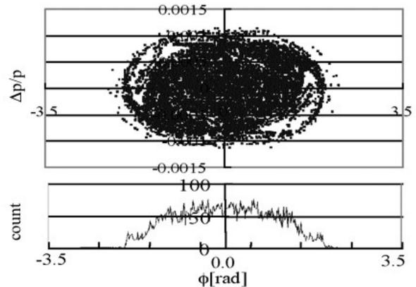
Figure 5: longitudinal phase space plot (top) and projection (bottom) at extraction. Harmonic number  $h=2$  and  $h=1$ .
