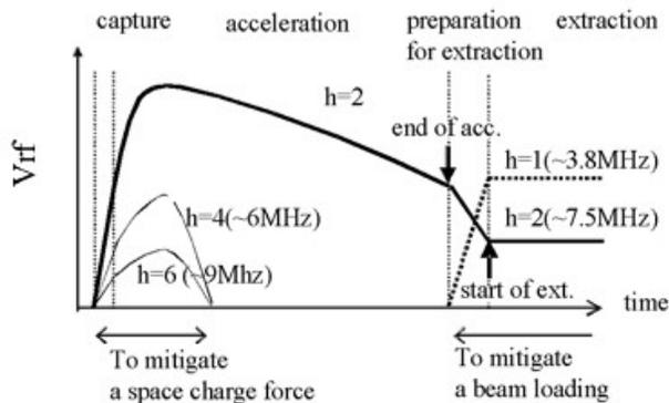
Figure 3: Schematic patterns of RF voltage for multiple harmonics operation.
