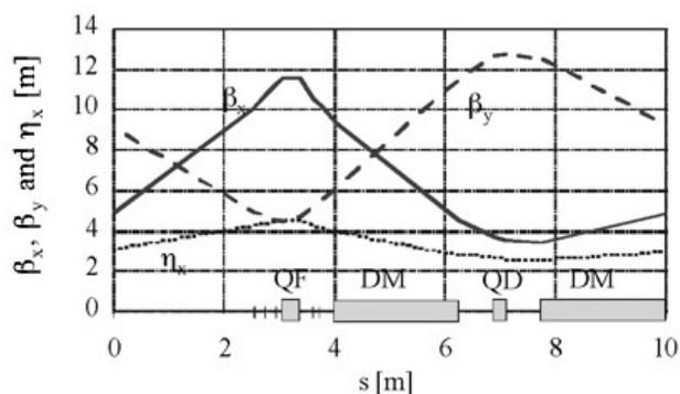
Figure 2: Beta and dispersion functions for one super-period.
