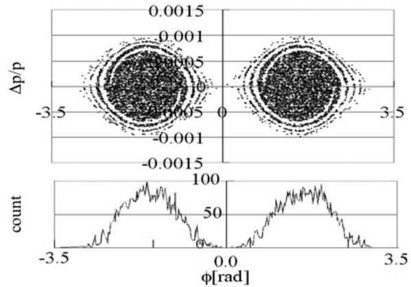
Figure 4: Longitudinal phase space plot (top) and projection (bottom) at extraction. Harmonic number  $h=2$ .
