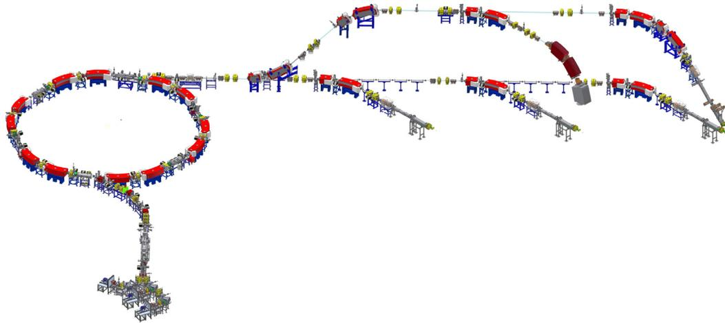
Figure 2: Possible layout of a particle-therapy accelerator, featuring three sources and three treatment rooms with horizontal, vertical and semi-vertical ( $45^\circ$ ) beam-ports, the last two rooms contain a dual beam-port each.
