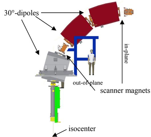
Figure 5: Layout of the last section of the vertical beamline.
