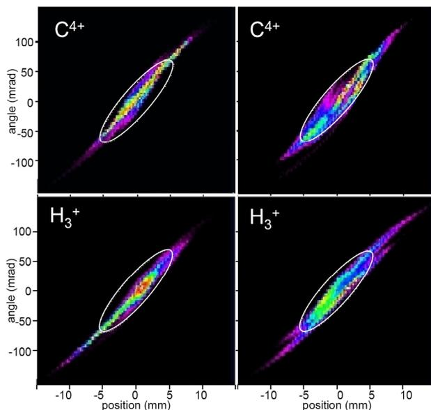
Figure 3: Emittances (left:horizontal, right: vertical) of  $C^{4+}$  and  $H_3^+$  beams at the end of the LEBT. The circumscribed emittances correspond to  $180 \pi \text{ mm mrad}$ , respectively
