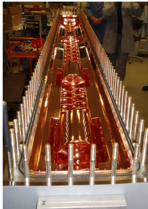
Figure 4: Inside view of the IH-DTL, showing the 4 accelerating sections, separated by quadrupole triplets.
