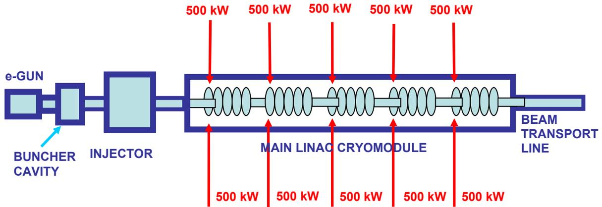
Figure 1: Schematic layout of 5 MW electron linac based on 704MHz SRF technology.
