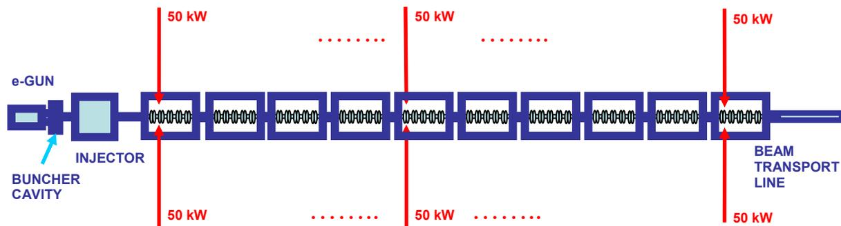
Figure 2: Schematic layout of 5 MW electron linac based on 1.3 GHz SRF technology.
