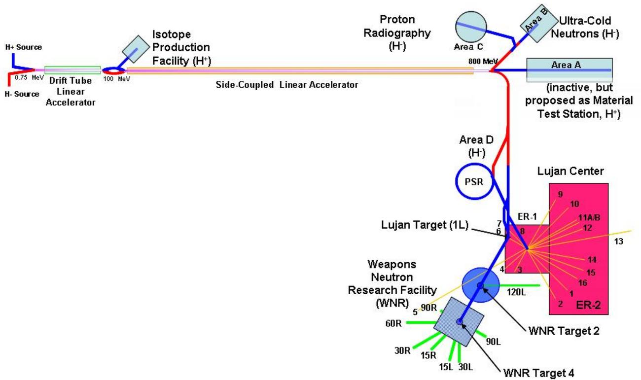
Figure 1: Schematic of the LANSCE Facility. The present Isotope Production Facility is shown in the upper left. WNR Target 2, where these experiments were conducted, is in the lower right. The Proton Radiography and Ultra-cold Neutron areas, which can run 800-MeV experiments while WNR runs 197-MeV experiments, are in the upper right.
