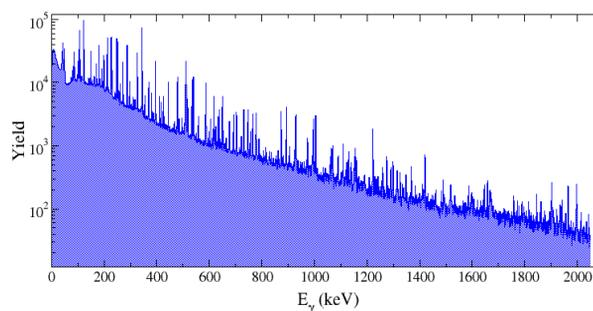
Figure 4: After irradiation, the Tb foils were taken to a counting station where the gamma decays were tracked with High Purity Germanium (HPGe) detectors. A spectrum from 30 minutes of counting approximately 12 hours after irradiation is shown above.
