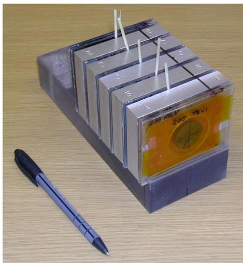
Figure 3: Shown above is the stack used for the sample irradiation. It consisted of 6 Tb foils, 5 Al degraders, and several Al beam monitors.
