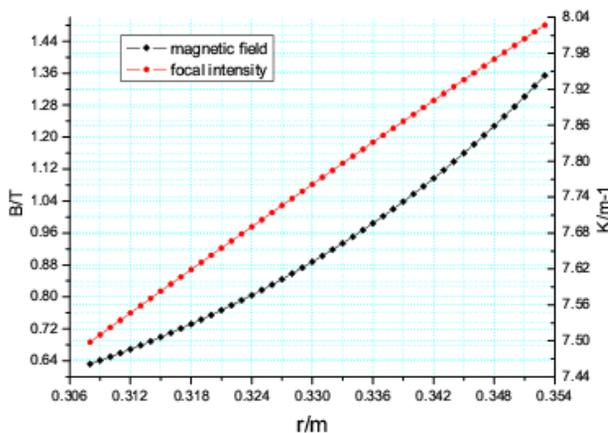
Figure 3: The changes of F magnetic field and focal intensity with the radius of curvature
