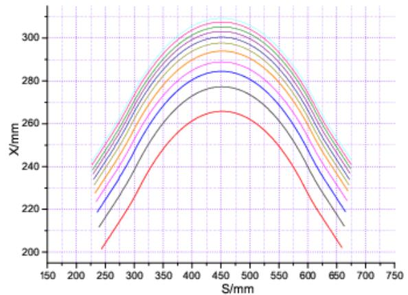
Figure 4: Closed orbit of one cell for different energies.
