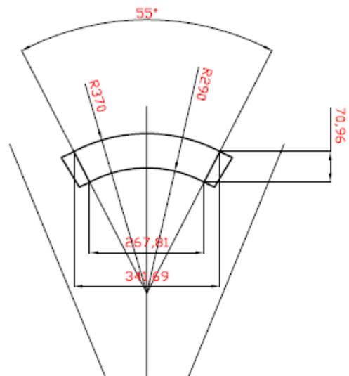
Figure 1: F magnet physical size of periodic structure.
