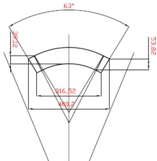
Figure 2: D magnet physical size of periodic structure.
