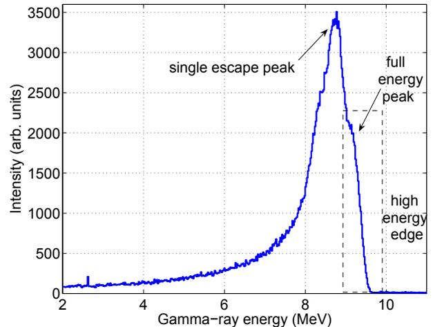
Figure 1: Measured energy spectrum of a gamma-ray beam produced by Compton scattering of a 466 MeV electron beam with a 789 nm Free-electron Laser beam at the High Intensity  $\gamma$ -ray Source (HI $\gamma$ S) facility. The gamma-ray beam is collimated by a lead aperture with a radius of 12.7 mm placed 60 m downstream from the collision point. After collimation, the gamma-ray beam is detected by a large volume 123% HPGe detector placed downstream 10 m from the collimator.
