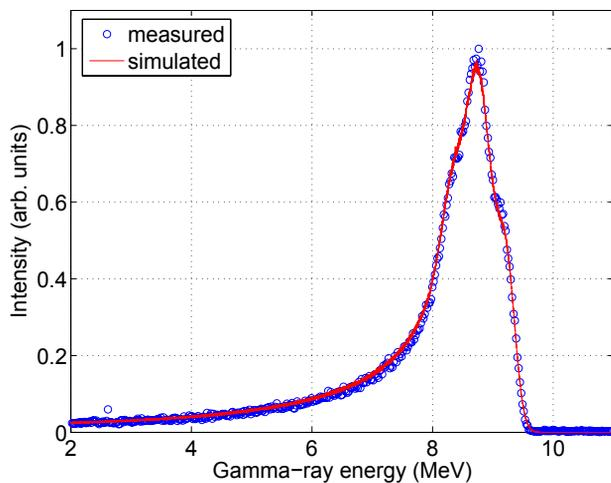
Figure 4: The simulated energy spectrum compared with the measured spectrum shown in Fig. 1.
