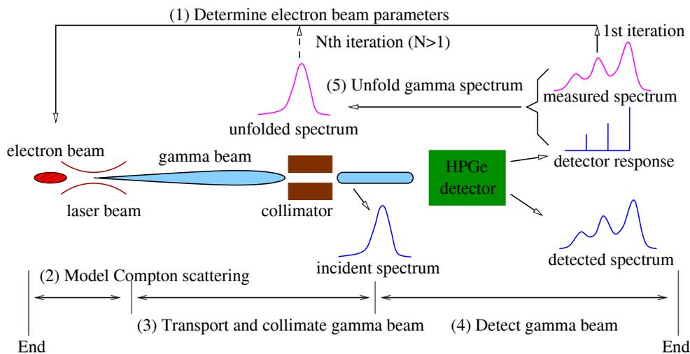
Figure 2: Illustration of the end-to-end spectrum reconstruction method to recover the energy distribution of a Compton gamma-ray beam. A few iterations are typically adequate to find a convergent energy distribution as well as the electron beam energy and energy spread.
