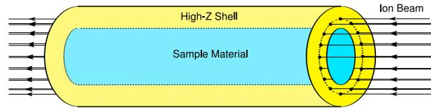
Figure 2: LAPLAS scheme using a beam with an annular focal spot.
