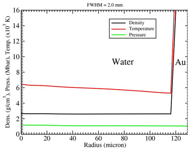
Figure 4:  $\rho$ , T and P vs radius in the water layer at the time of maximum compression for a beam FWHM = 2 mm.
