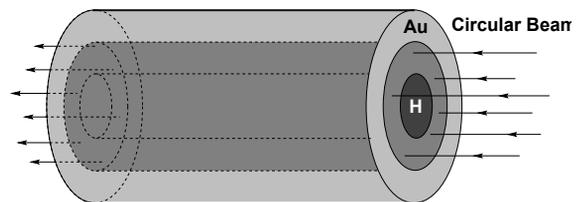
Figure 3: LAPLAS scheme using a beam with a circular focal spot.
