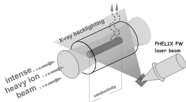
Figure 1: HIHEX scheme using a solid cylindrical target.
