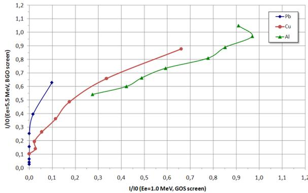
Figure 5: Transmission of the HE beam as detected by BGO versus transmission of the LE beam as detected by GOS.
