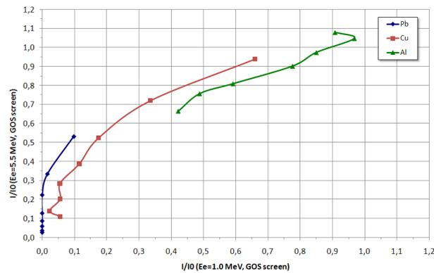
Figure 2: Transmission of the HE beam versus transmission of the LE beam. GOS scintillator.
