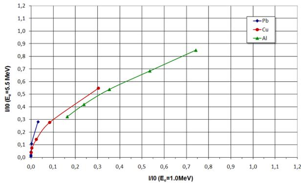
Figure 1: Transmission of the HE beam versus transmission of the LE beam. Ideal detector.
