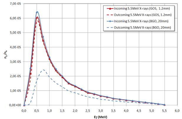
Figure 4: Incoming and outgoing x-ray spectra for GOS (1.2mm) and BGO (20mm) scintillators.  $E_e = 5.5 MeV$ .
