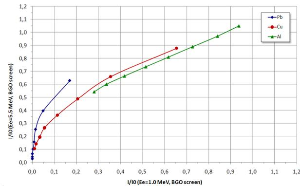
Figure 3: Transmission of the HE beam versus transmission of the LE beam. BGO scintillator.
