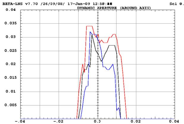
Figure 3: Dynamical aperture for on (black) and off momentum (+3% blue and -3% red) at injection point.
