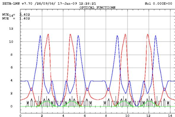
Figure 2: Horizontal (red), and vertical (blue) beta functions.
