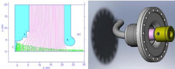
Figure 3: Shape of the injector. C is the cathode, F is the focusing electrode, A is the anode, which is the wall of first accelerating cell AC of the accelerating section. Z is the accelerating section axis.
