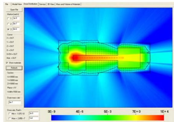
Figure 5: Calculated dose rate (Rad/sec) distribution (black line is 8·10<sup>-6</sup> Rad/sec isodose).
