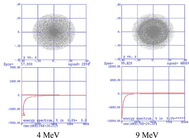
Figure 2: Beam cross-section and electron energy spectra for 4 and 9 MeV.
