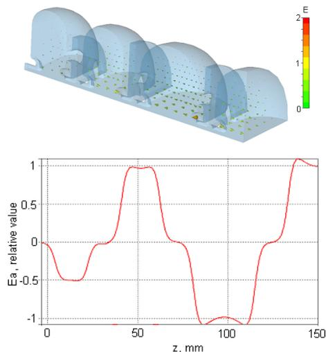
Figure 1: Calculation model and accelerating field distribution in first three and half accelerating cells.
