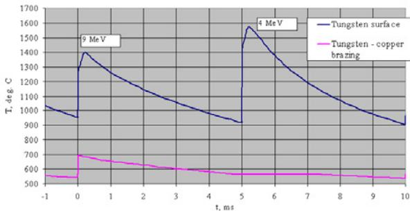
Figure 4: Temperature distribution versus time on the Tungsten (blue) and Tungsten-Copper brazing surfaces (pink).
