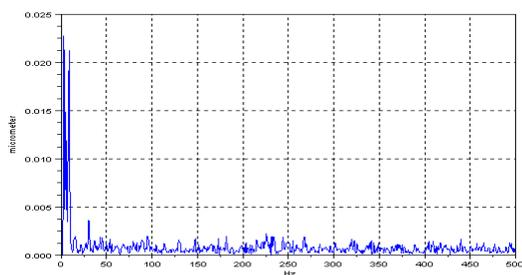
Figure 9: spectrum of the rotational stage mounted on the optical table [4].
