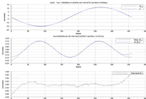
Figure 4: One-turn data and the fitting result with sine wave.
