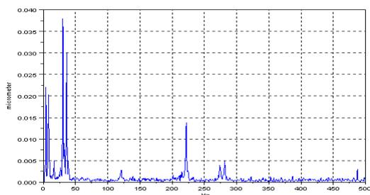
Figure 10: spectrum of the rotational stage mounted on the X-Y table.
