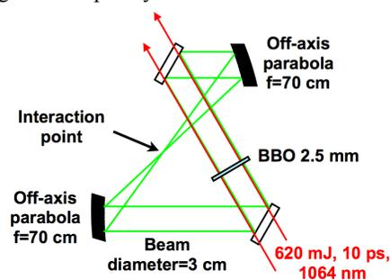
Figure 1: RING pulse recirculator
