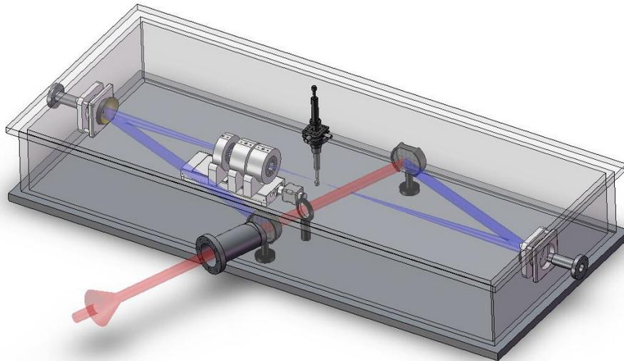
Figure 2: CAD rendering of the interaction region showing a simplified vacuum chamber, the laser path through the RING optics, PMQ final focus assembly, and diagnostic cube.
