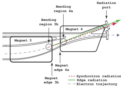
Figure 2: Diagram of the last two magnets of the chicane, showing sources of the radiation that was collected.
