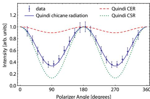
Figure 5: Chicane radiation polarization from measurement and QUINDI simulation; also shown are QUINDI simulations of single magnet CER and CSR.
