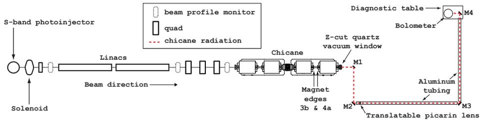
Figure 1: Diagram of the relevant beamline section and chicane radiation transport.
