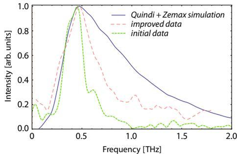
Figure 4: Measurements of the chicane radiation spectrum before and after transport line improvements were made, compared to start-to-end simulations. The simulated spectrum is broader due to the fact that QUINDI does not model self-fields, which increase the energy spread and result in a longer bunch and thus a broader spectrum.
