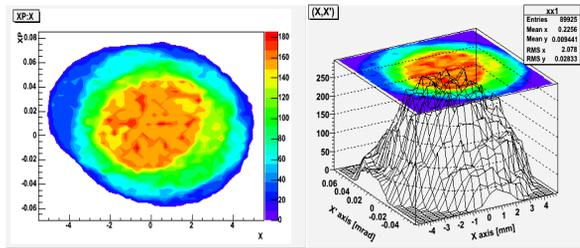
Figure 2: Transversal painting in  $(x,x')$  during 5 turns.
