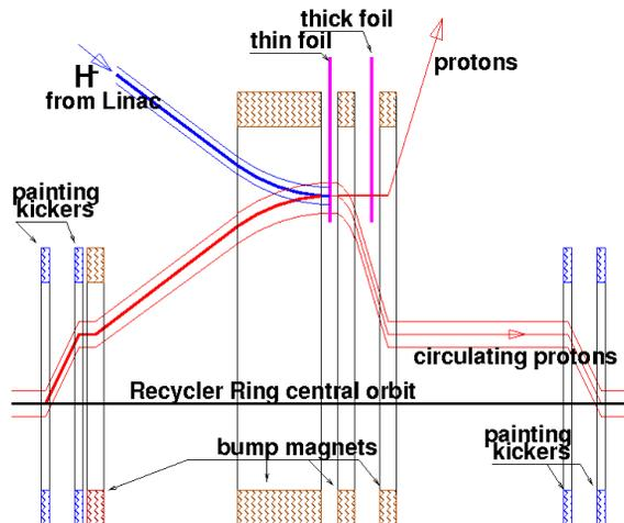
Figure 1: Injection chicane layout.
