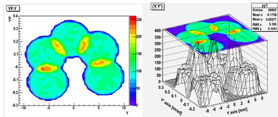
Figure 3: Transversal painting in  $(y,y')$  after 5 turns.
