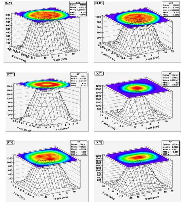
Figure 4: Phase space distributions during transversal painting with zero (left) and full (right) space charge after 500 turns.
