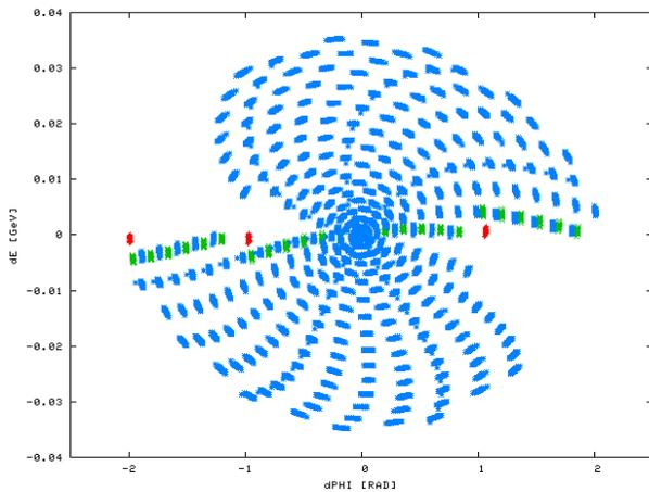
Figure 6: Longitudinal painting mechanism  $\Delta\phi$  [mrad] (horizontal),  $\Delta E$  [GeV] (vertical). Microbunches, injected from linac, after 1 turn (red), after 6 turns (green) and after 77 turns (blue).
