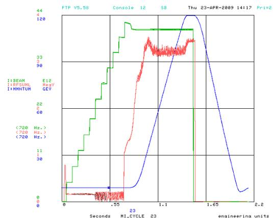
Figure 2: The total intensity (green), rf voltage (red) and momentum in the MI (blue) on the mixed mode cycle.
