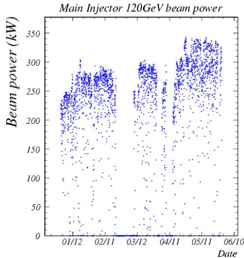
Figure 3: The total beam power of mixed mode cycle from January to July 2008. Plot shows before and after the 11 batch slip stacking process became operational.
