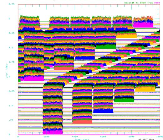
Figure 1: Mountain range plot showing the 11 batch slip stacking process in the mixed mode cycle. Horizontal scale is a MI revolution of  $\sim 11 \mu\text{sec}$ .
