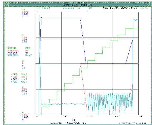
Figure 4: The frequency functions for the first rf system (red) and the second rf system (blue), the total rf voltage (cyan), and the beam intensity (green) in the MI.
