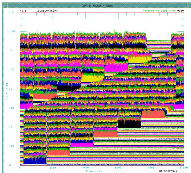
Figure 5: Mountain range plot showing a 12 batch slip stacking process at 8 GeV in the MI. Horizontal scale is a MI revolution of  $\sim 11$   $\mu$ sec.
