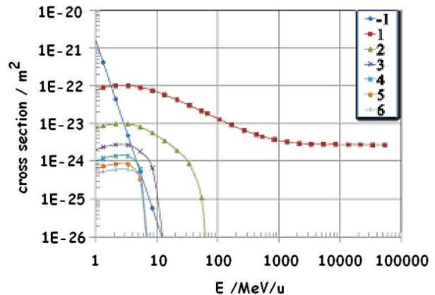
Figure 4: Cross section for different degrees of ionisation in H.
