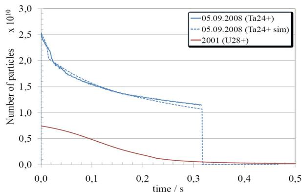
Figure 6: Time dependent intensity of intermediate charge state heavy ions (Ta<sup>24+</sup> and U<sup>28+</sup>) in a SIS18 cycle. The significant amount of beam loss is due to charge changing processes – mainly ionization. The progress as indicated by the two intensity curves has been made in the frame of the SIS18upgrade program.
