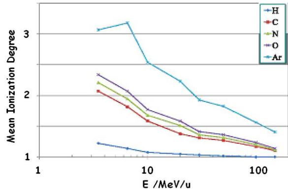
Figure 3: Mean ionisation degree increase for  $U^{28+}$  as a function of the beam energy.
