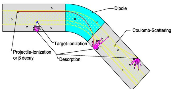
Figure 1: Electron capture or ionization processes at collisions with residual gas atoms and molecules change the charge state of the beam ions. Gas desorption drives a pressure bump at the impact position after dispersive elements.
