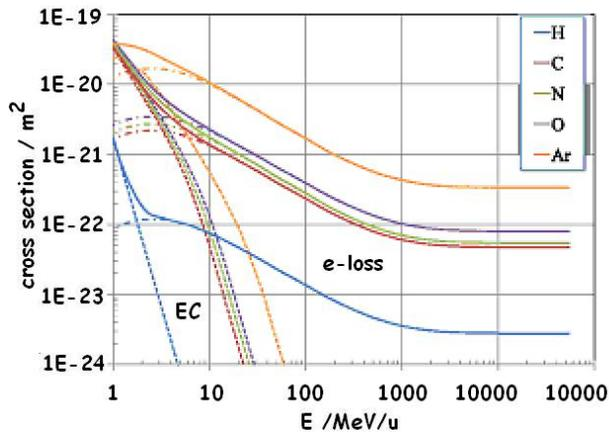
Figure 2: Electron capture cross section (short dashed lines), loss cross sections (long dashed lines) and total cross section (solid line) for charge change of  $U^{28+}$  as a function of the beam energy.
