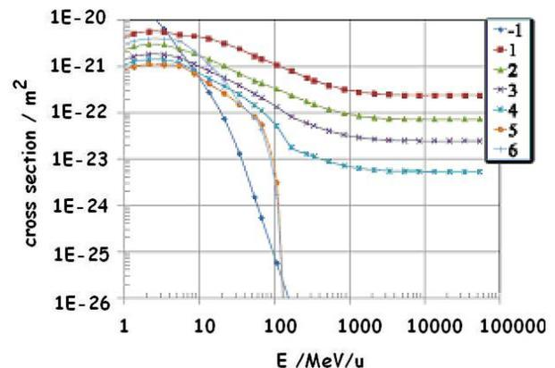
Figure 5: Cross section for different degrees of ionisation in Argon.
