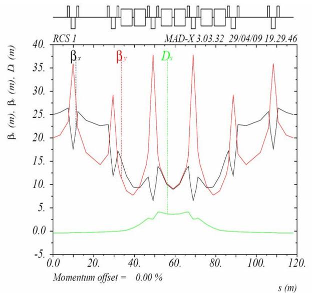
Figure 3: Betatron functions of the 6.4 (10.3) GeV RCS for the Neutrino Factory.
