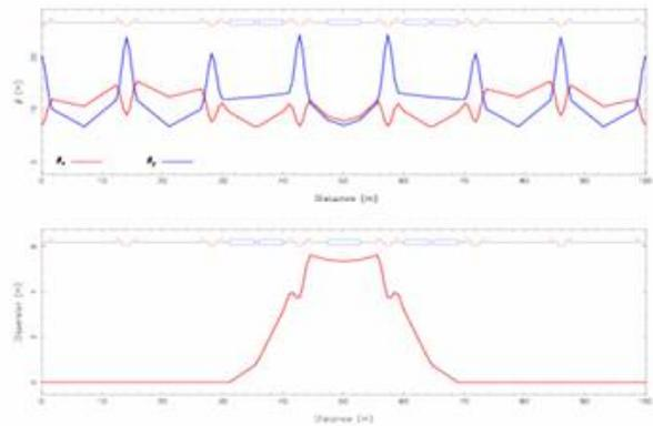
Figure 1: Betatron functions in the 3.2 GeV RCS for the ISIS upgrade.
