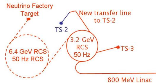
Figure 2: Conceptual layout of the common proton driver for the neutron spallation source and the Neutrino Factory based on ISIS upgrade. The solid lines show a facility studied in the framework of the MW ISIS upgrade, the dashed ones show the part which needs to be added in order to supply the Neutrino Factory.
