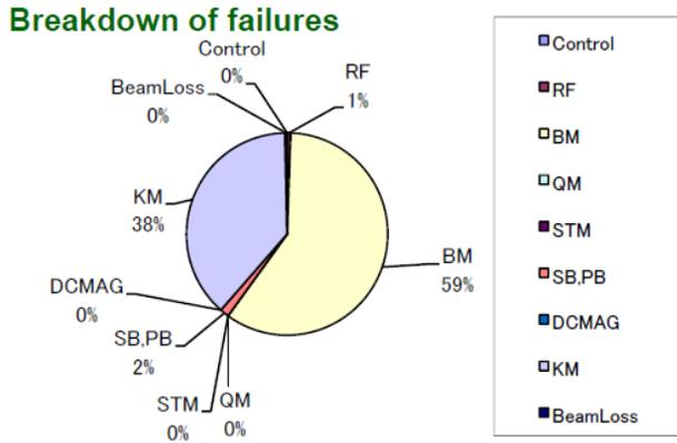
Figure 1: Breakdown of failures of RCS after user operation. Failures were mainly caused as follows, RF: "OC/UV" interlock of the screen grid, KM: pre-fire of Thyatron for extraction kicker magnet, SB&PB: power supply was down by the noise, and BM: troubles.
