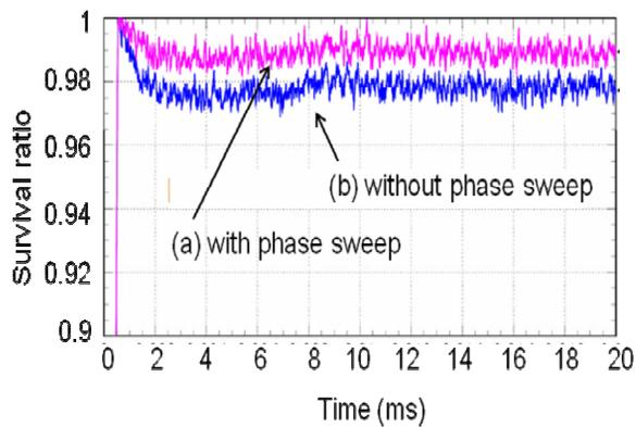
Figure 3: DCCT signal in high power demonstration. The beam condition is as follows, H- peak current is 15 mA, pulse length is 0.5 ms, intermediate-pulse width is 600 ns, bunch number is 2, transverse painting is done with  $15 \pi$  mm mrad for both horizontal and vertical, and also longitudinal painting is done with 80% of 2<sup>nd</sup> harmonics is added and -0.1 % momentum offset. (a) phase-sweep from -80 to 0 degree, (b) without phase-sweep.
