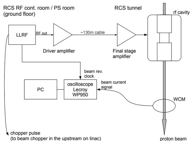
Figure 1: Beam test setup.
