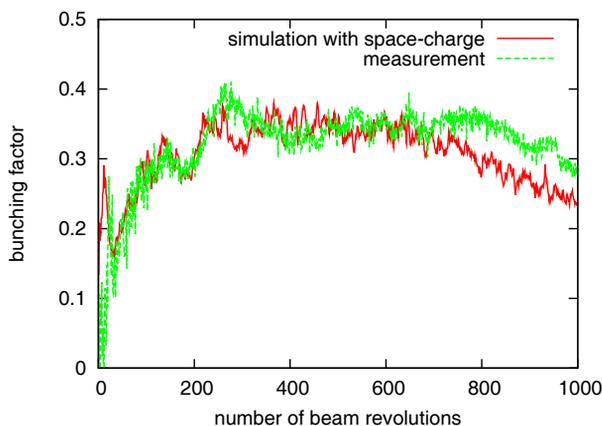
Figure 4: Comparison between the simulation and the measurement, with 80 % second harmonic, momentum offset of  $-0.2\%$  and phase sweep of 80 degrees.
