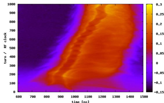
Figure 5: A mountain plot of the high current operation.  $2.932 \times 10^{13}$  protons, which correspond to 352 kW at 25 Hz operation, are successfully accelerated.
