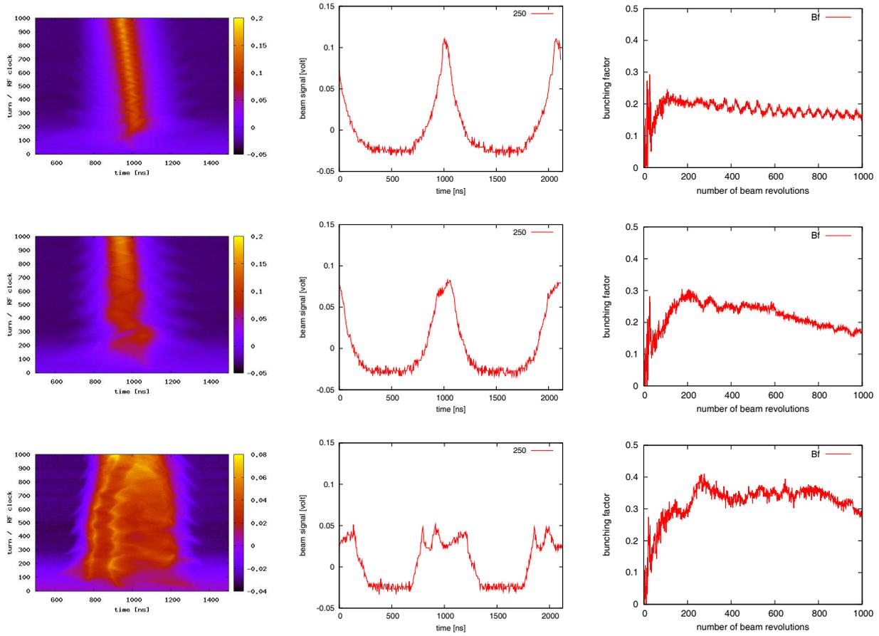
Figure 3: (Left) Mountain plots, (center) bunch shapes at 250-th turn, and (right) Bunching factor plots, in the cases of (upper) (i) fundamental RF only, (middle) (ii) with 50 % second harmonic, (lower) (iii) with 80 % second harmonic, momentum offset of  $-0.2\%$  and phase sweep of 80 degrees.
