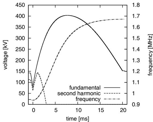
Figure 2: Accelerating voltage program with 80 % second harmonic and frequency program.  $t = 0$  corresponds to  $B_{min}$ . The beam is injected from 117 turns before  $B_{min}$  to 117 turns after  $B_{min}$ .
