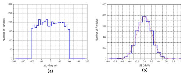
Figure 8: Uniform and Gaussian distribution with  $\sigma_E = 200$  keV in (a)  $\Delta\phi$  and (b)  $\Delta E$  spaces.
