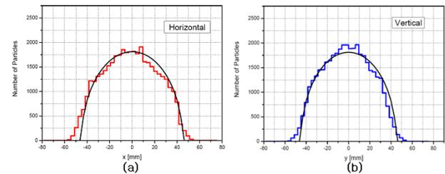
Figure 4: Particle distribution in (a) horizontal and (b) vertical directions.
