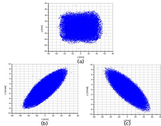
Figure 3: Particle distribution after injection in (a)x-y space, (b) x-x' space, and (c) y-y' space.
