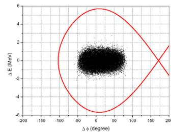
Figure 10: Particle distribution in the RF bucket after acceleration process.
