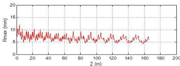
Figure 8: Beam envelope for the alternative accelerating lattice from  $\sim 156$  MeV to 1.2 GeV.
