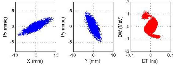
Figure 4: Horizontal (left), vertical (middle) and longitudinal (right) phase space after the matching section of the alternative accelerating lattice, at a beam energy of  $\sim 156$  MeV.
