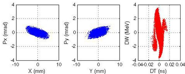
Figure 9: Horizontal (left), vertical (middle) and longitudinal (right) phase spaces at the exit of the alternative lattice, at a beam energy of  $\sim 1.2$  GeV.
