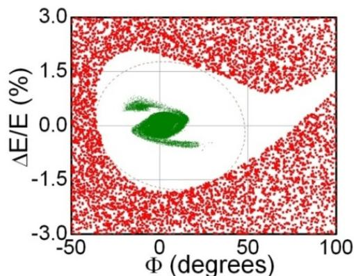
Figure 7: Longitudinal acceptance of the 1.3 GHz elliptical accelerating structure at  $\sim 156$  MeV (white) together with the matched input beam phase space (green).
