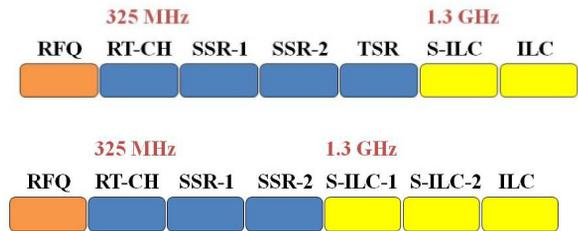
Figure 1: Project X baseline linac (above) and the alternative linac layout (bottom).
