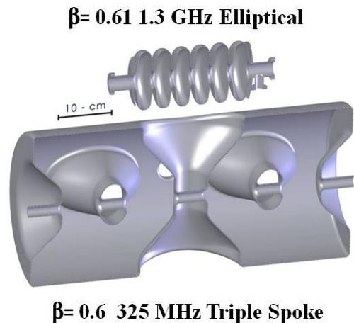
Figure 2: 1.3 GHz  $\beta = 0.61$  Elliptical structure (top) and 325 MHz  $\beta = 0.6$  Triple-Spoke structure (bottom).
