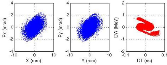
Figure 3: Horizontal (left), vertical (middle) and longitudinal (right) phase spaces at the exit of the SSR2 segment in the baseline linac, at a beam energy of  $\sim 126$  MeV.
