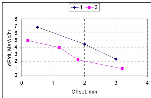
Figure 4: Comparison of the longitudinal cooling rates at various vertical offsets of the electron beam before (set 2) and after (set 1) adjustments of quadrupoles. Antiproton beam parameters for set 1/set 2: number of antiprotons 100/61  $10^{10}$ , beam length 5.5/4.1  $\mu\text{s}$ , transverse emittance measured with a flying wire 2.6/3.8  $\pi$  95% normalized, rms momentum spread 3.2/3.5 MeV/c.
