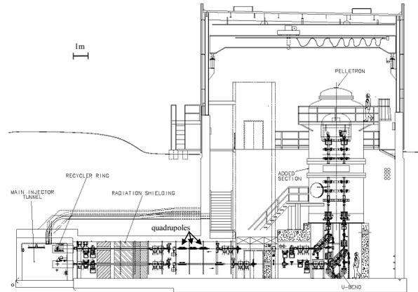
Figure 1a: Elevation view showing the Pelletron with its acceleration and deceleration tubes, the transfer lines passing through the connecting enclosure to the Recycler ring, and the cross-section of the Main Injector tunnel which houses the Recycler ring.
