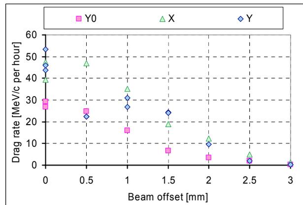
Figure 3: Drag rate as a function of the offsets between the antiproton and electron beams. The set labelled Y0 represents data recorded for vertical offsets before applying the quadrupole correction. The sets X and Y show the results after quadrupole correction for offsets in horizontal and vertical directions, correspondingly.
