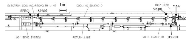
Figure 1b: Elevation view of the Main Injector tunnel showing the 90°-bend system which injects the electron beam from the transfer line into the Recycler ring, the cooling section of Recycler, the 180°-bend system which extracts the electron beam from the Recycler, and the return line. BYR01 labels the BPM in a high-dispersion location, which is used for energy measurements and stabilization.
