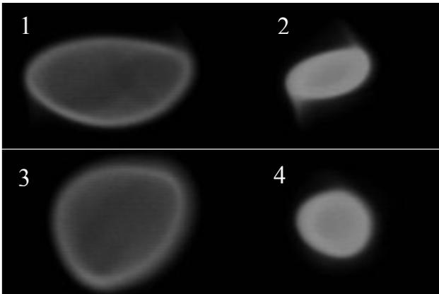
Figure 2: Images of the beam at the YAG with zero (1 and 2) and adjusted (3 and 4) quadrupole currents. Images were recorded at zero current of the lens SPQ01 (1 and 3) and at 10.4 A (2 and 4). All other settings are the same for all images. Beam current was 0.1 A, the pulse duration was 2  $\mu$ s, and the camera was gated over a 100-ns window at the peak of the pulse.
