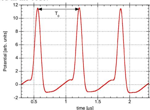
Figure 3: Potential of the synchrotron motion in the barrier bucket. The valley in the potential is due to a small bank of the voltage between the sinusoidal boundaries [4]. Here a large fraction of the particles can be captured if the momentum spread is sufficiently cooled down.
