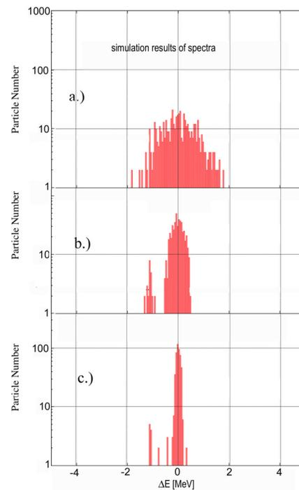
Figure 4: Predicted beam spectra at initial time (a.), after 60 s (b.) and after 160 s (c.). Stochastic cooling and target are switched on.
