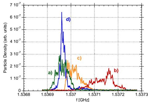
Figure 2: Schottky spectra of a COSY proton beam measured at the 1000<sup>th</sup> harmonic: a) initial distribution; b) final distribution after 160 sec only pellet-target, the energy loss led to a shift to higher frequencies since COSY was operated above transition; c) final distribution with longitudinal stochastic cooling only and d) final distribution with cooling and barrier bucket. The mean energy loss is compensated. Data are taken from ref. [4].
