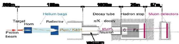
Figure 1: Schematic layout of the CNGS secondary beam.
