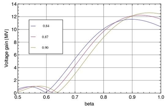
Figure 4: Voltage gain for the different  $\beta_g$  cavities, where  $\phi_s = 0$ .
