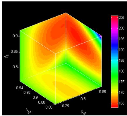
Figure 3: Total number of  $\{\beta_{g1} + \beta_{g2}\}$  cavities required to accelerate the beam between 450 MeV and 2.2 GeV. A minimum of 165 is required for  $\beta_{g1} = 0.82$ ,  $\beta_{g2} = 0.94$ , and transition  $\beta = 0.86$ .
