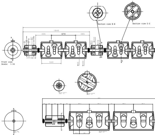
Figure 1: Upper frame: Super-ferric quad doublet and  $\beta_g = 0.35$  DSR cavity layout. Bottom Frame: Super-ferric quad doublet and  $\beta_g = 0.59$  TSR cavity layout.
