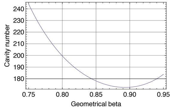
Figure 2: Number of 5 cell cavities required to accelerate the beam between 450 MeV and 2.2 GeV as a function of  $\beta_g$ . A value of  $E_o$  of 25 MV/m and a synchronous phase of  $-25^\circ$  have been assumed.
