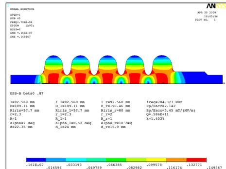
Figure 5: Relative electric field intensity of the designed  $\beta_g = 0.87$  structure.
