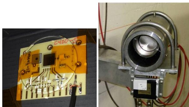
Figure 3: Left: the pCVD board with the detector sensor. Right: the detector assembly with the ACEM PMT on top in its shielding and the pCVD detector at the bottom.
